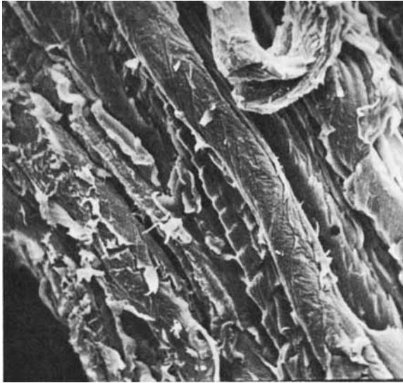
Fig. 5. Surface topology of 109% PMMA grafted sisal fibers, \times 480 .
