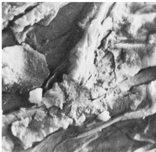
Fig. 4. Surface topology of 20% PMA grafted sisal fibers, \times 1500 .
